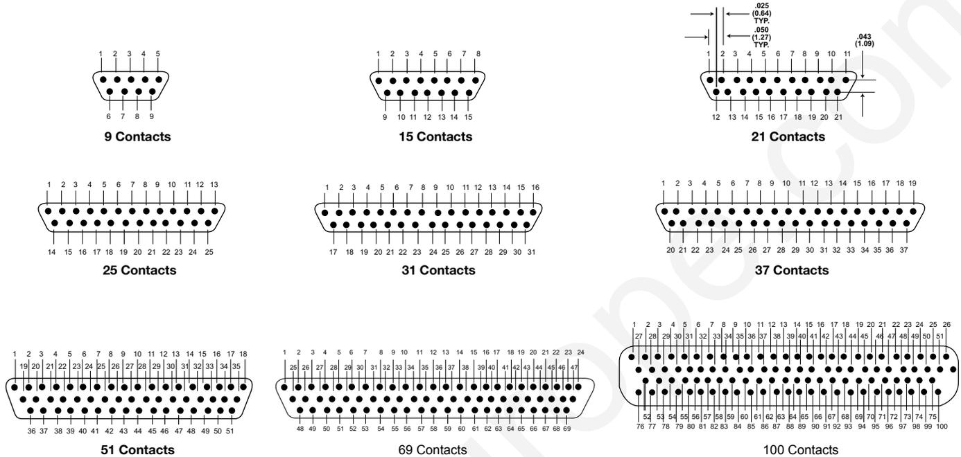
Contact identification numbers are for reference only and do not appear on insulation or connector body.
