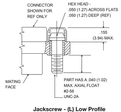
Shown here is a cutaway view of the float mount for the MD connector. The basic shell dimensions are the same for the float mount and the screw mounting hole configurations. View shown is for standard float mount front panel mounting. Reverse mounting is available on request.
