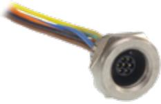
Cannon's MIKQ Microminiature Circular Connectors feature a quick disconnect metal shell and a receptacle version that, when engaged, can be instantly disconnected while still providing a solid lock. Applications include commercial TV cameras, portable radios, military gun sights, airborne landing systems and medical equipment. Maximum temperature range is -55°C to +125°C.
