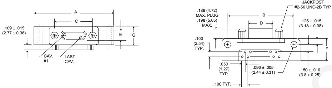
PCB Termination Arrangements (Viewed from bottom of connector, PCB solder side.)
