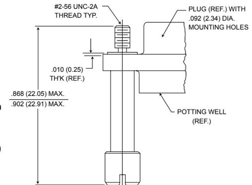
**Figure 2. Jackscrew - High Profile Slotted Head**
