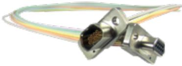
The Ultra-High Temp Micro-MDM series is qualification tested to withstand 230°C continuous operating temperature for 500 hours and meets the harsh requirements of the Oil and Gas exploration industries. Cannon's Ultra-High Temp Micro-MDM F300 connector is designated by an F300 modification code and uses high performance Micro Twist Pin Contacts, special insulating materials and high temperature wire.
