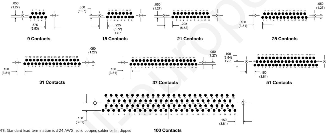
NOTE: Standard lead termination is #24 AWG, solid copper, solder or tin dipped
