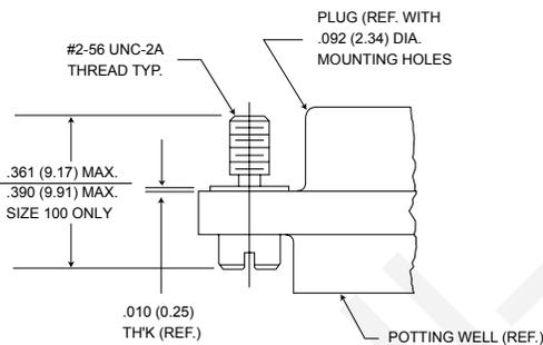
**Figure 1. Jackscrew - Low profile Slotted Head**
