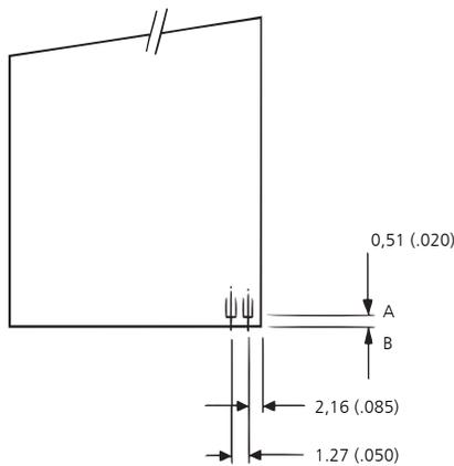
**Diagram 1** shows details of the pad spacing and the suggested amount of material to be left between the end of the pad A and the edge of the flex B.
