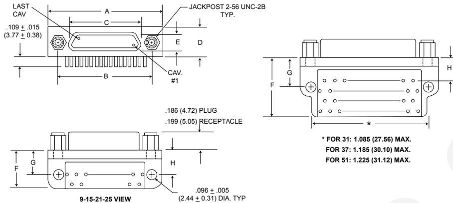
PCB Termination Arrangements (Viewed from bottom of connector, on PCB solder side.)
