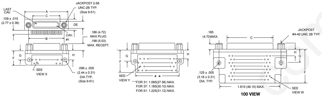
PCB Termination Arrangements (Viewed from bottom of connector, PCB solder side.)
